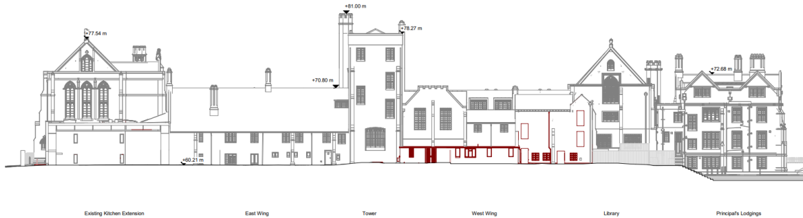
1 North Range - North Elevation - Demolition 1:200
